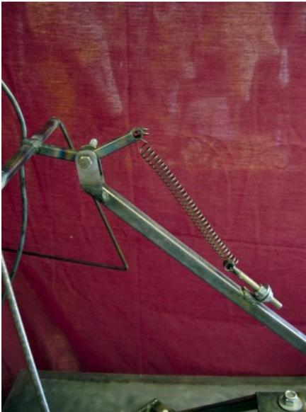
The end of the lift arm is angled up to accept the prop torso/character. The degree of this angle must be greater than the lift arm's fully extended arc angle so the prop body doesn't come in steady contact with the arm.
