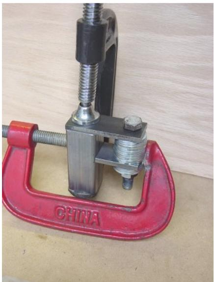
This is the swing cylinder clevis mount bracket clamped for welding. Same procedure, different configuration.
