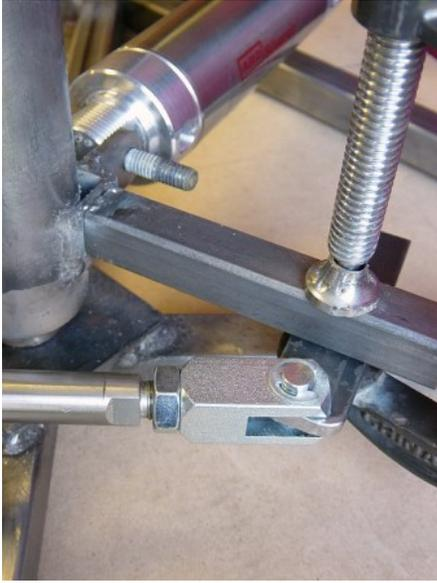
With the cylinders and their mounting brackets connected, it's easy to clamp the brackets to linkage components for test fitting. Clamp each end securely and manually move the part. If needed, reposition the mounting bracket and test again. Once satisfied with the joint's range of motion and acceptable clearance(s) it's safe to tack the mounting brackets in place. Remove the clamps and test the motion again.
