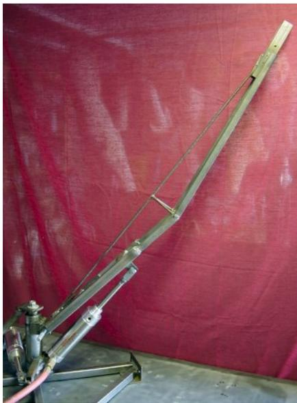
Parallel lower bars provide most of the linear strength for this arm assembly. By running them side-by-side, chances of side flexing are greatly reduced. The dual lower arm bars are angled near midpoint to lay parallel the ground as much as possible. This low profile characteristic should aid in reducing the apparent size of the whole prop when at rest.
