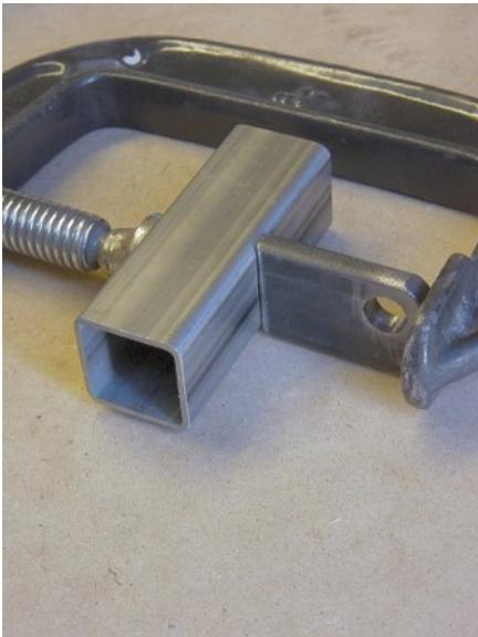
This "tee" shaped bracket will be welded to the lift arm. This is made of 1 inch square tube cut to proper length and 1" X 1/4" flat bar drilled and cut to length. This hole will be used to attach the cylinder's rod end clevis to the lift arm.
