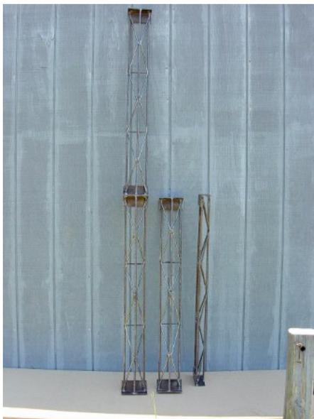
The lengths of rebar are tacked in place between two angle pieces. Check for straight and square, and weld them in place.
