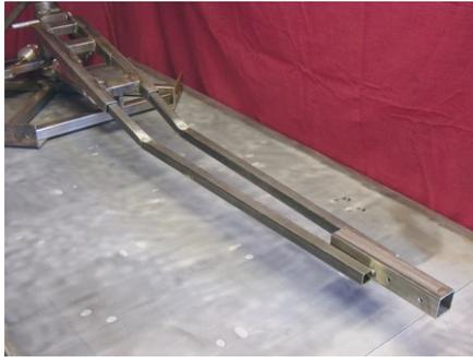
As previously mentioned, the lift arm for this machine will be fairly long. Any combination of substantial weight and sudden changes in motion would cause a long, thin arm member to flex. To eliminate this flex without using a heavy walled single tube (which would add even more weight at the end of the arm) I decided to break the arm into two segments.
