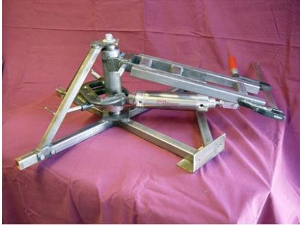
The shop made cylinder mounting brackets are installed on the air cylinder and clamped in position on the machine.
