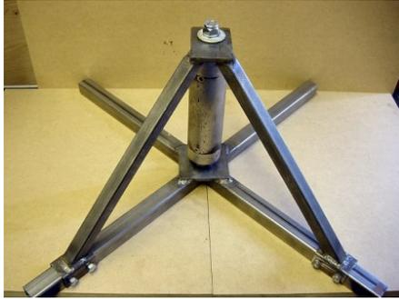
Rear braces are added to keep the spindle assembly securely in position.
