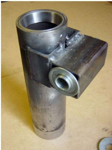
Considering the desired strength of this joint, the 1/2" i.d. is perfectly suited to a 1/2 pin. Anything smaller might not be strong enough if the prop weight and leverage become larger than anticipated. The bearing's outer diameter is slightly larger than the inside measurement of 14 gauge 1 1/4" square tube. This worked out perfectly. The bearings were pressed in and remain snugly in place.
