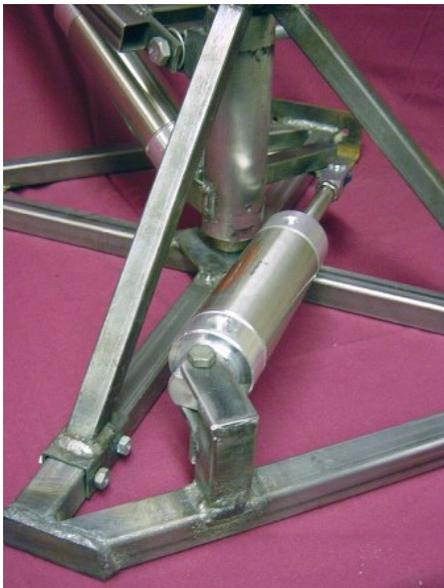
Finished and mounted swing cylinder assembly, mounting brackets, etc.
