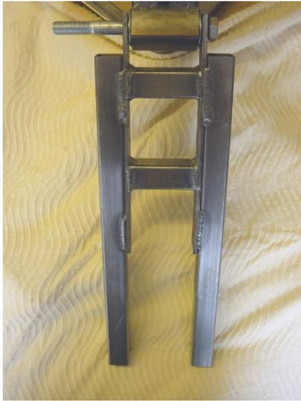
This is the base section of the lift arm. This mounts to the pivot joint attached to the spindle.
