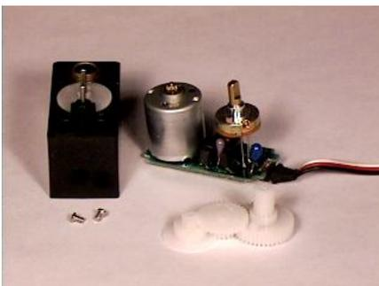
Connecting the SERVO to a controller is fairly straightforward. SERVOS have a 3-wire connector. One RED wire(for power), one BLACK wire(for ground) and a WHITE or YELLOW wire(for control). The first two wires are pretty self explanatory, but I feel it necessary to explain the control wire a little further.
