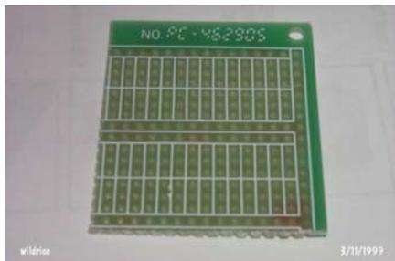
If you look at the board, it is arranged the same as a solder less bread board. This allows you to lay out things on the breadboard, then transfer them directly to the PCB. In this case, the circuit is so simple, that we can just solder it up.
