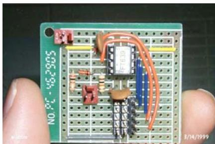
This is the board with the parts in place, ready to be soldered. The blue and orange lines are the servo signal lines. The 3 by 5 array of pins is where you plug the servos in. The center column of 5 pins all carry +5 volts. The left 5 are all ground, and the right 5 are the 5 servo signal lines. Each servo uses three pins, ground, +5, and one of the signal pins.
