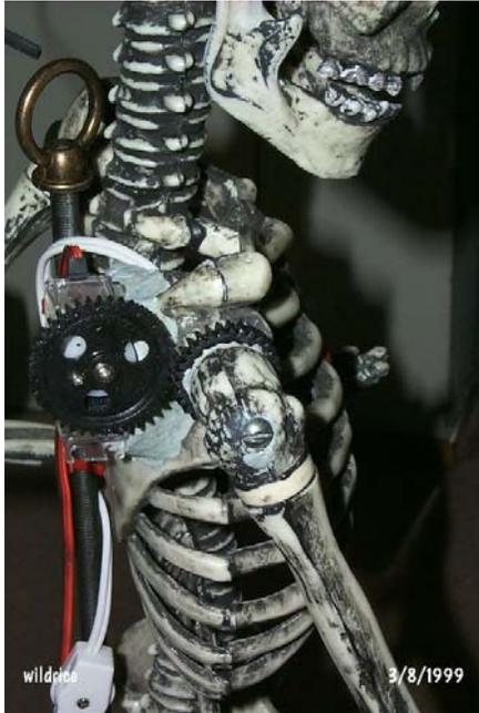
The side view shows the gears used to move the shoulder. The small gear is attached directly to the arm. It is driven by the larger gear which is attached to the servo. The servo is connected to the skeleton with epoxy.
