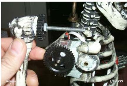
To animate the arm, I broke it off at the movable joint (that takes guts!), then I drilled out the joint and filled it with [putty epoxy](#) (there are several brands available from most hardware stores, any will do. ). Before the epoxy hardened, I inserted a 3 to 4 inch stove bolt and positioned it correctly, then packed the putty around it. Once the epoxy had hardened (full cure in about half an hour), I threaded a small gear (T30) that
