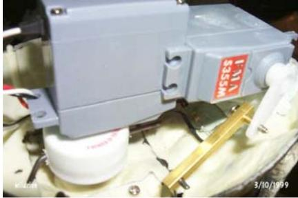
This is another view of the skull servos. Here you can see that the bottle cap is pinned to the neck by drilling a hole through it and the neck and inserting a pin. The bottle cap is bigger than the neck which allows it to float. That way, even if the servo and the neck are not aligned exactly, they still work well together as the neck is free to move small amounts along the pin as the skull turns.
