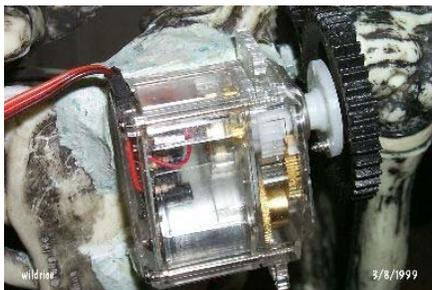
Next I took a [CIRRUS CS-60BB](#) servo I purchased from [Sheldon's Hobby](#) for \$24.99 and replacing the short center screw with a longer one from the servo parts pack, I attached a T40 gear (from the same 5 pack I got above) to the servo horn (the white piece). I drilled a small hole for an additional screw to tie the servo horn and the gear together.
