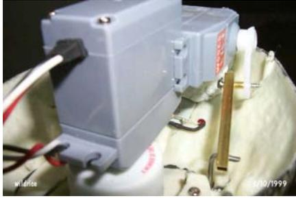
Here are the servos mounted inside the skull. The jaw servo is connected to the jaw lever (piano wire) with a piece of square brass tube with a hole drilled in either end. When I took this picture, I had a spacer between the control horn and the brass link, but I later removed it to make things align better.
