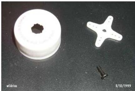
To connect the servo to the neck, I used a 2-liter pop bottle cap and a control horn. I hacked a hole into the top of the cap, then I glued the control horn inside the cap with some putty.
