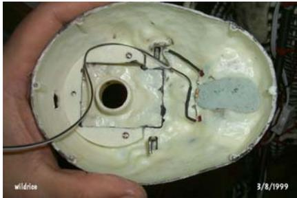
This is the inside of the skull. If you look hard, you can see the piano wire sticking up out of the jaw hinge near the bottom of the picture. You can also see the wiring of the LEDs for the eyes.
