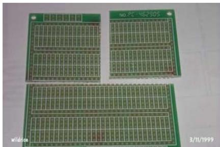
The SYNTAX PCB board is a good quality board and is relatively inexpensive. I generally keep several around. In this case, I want to put the board inside the Skull, so I cut the board (tin snips) and will only use one corner. The two smaller pictures are the front and back of the corner I chose. After cutting the PC board, take the small piece of sandpaper that comes with the epoxy putty and sand the edges and the board will be much nicer to work with.
