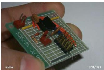
Here is the board at a different angle. You can see the two 0.1µf (104) [capacitors](#) better here. These caps absorb any noise from the power lines.
