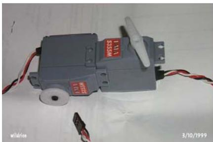
I glued the two servos that fit into the skull together with some thick super glue. The round control horn gets removed and replaced with the bottle cap I prepared above. I then cut one side of the lever control horn off. This servo controls the jaw.
