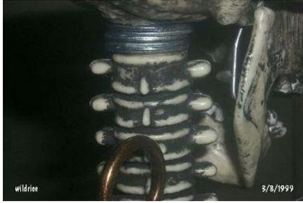
When the servos turn the head and the jaw opens and closes, the jaw hits the collar bone. To reduce this problem, I added metal washers on the neck to lift the skull up a bit higher so that when the jaw opens, it will clear the collar bone. Three washers are not quite enough, but any more and the neck does not protrude into the skull enough for control.
