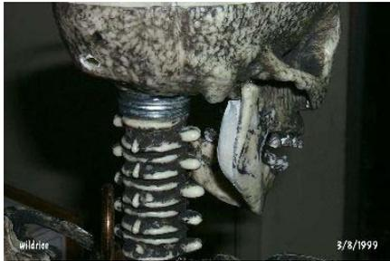
I then covered the piano wire with putty epoxy to prevent the wire from moving in relationship to the jaw when the servo pushed or pulled the wire. This makes the jaw movement much more exact.
