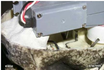
It is a bit hard to see since it is off white, but if this picture shows the putty that I used to form a mounting platform for the servos. I just mixed up a batch of putty, put it in place, then pushed the servo into it until it was in the right position. A few minutes later it was solid and hard.
