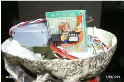
Now we are ready to mount the board. The side of the servo looked like a likely place, so I mixed up a tiny bit of putty epoxy and rolled it into four pea sized balls and stuck them to the side of the servo. Then I pressed the finished PC board into them.
