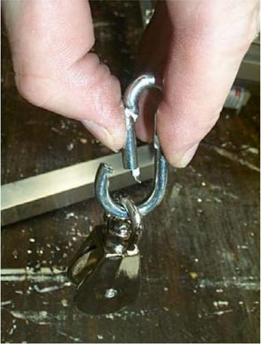
Now you can connect the swivel pulleys using the quick connects.
