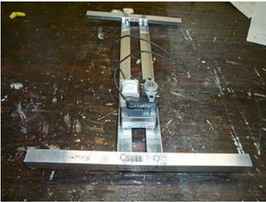
Use your (4) #10 X 1/2" bolts to secure the motor to the frame and tighten. Now you can go around and tighten all the other bolts/nuts and the frame will be nice and rigid. Do not over tighten or you will bend and flex the Aluminum and put extra stress on the little motor mount bolts.
