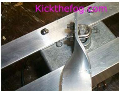
Put the nuts on and tighten them up. You'll notice in this picture that I have yet to tighten the nuts so there is a lot of space between the drive shaft and the inside of the u-bolt.
