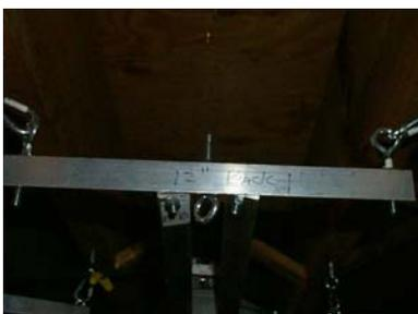
Now drill a 1/4" hole in the center of the 12" rear and install an eyebolt facing down. Do this in the exact same way that you've done the others. This will support the ghost.
