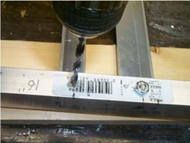
AN EASY WAY TO MARK AND DRILL these is to only drill the Front (top) piece first. Then use a screw or punch to make a mark for drilling. Do this by inserting a screw or punch into the top hole you just drilled and use a hammer to hit the screw or punch. This will make a mark on the aluminum underneath and give you a great mark as to where to drill. This way you do not have to try and drill all the way through BOTH pieces and have them jumping all over the place.
