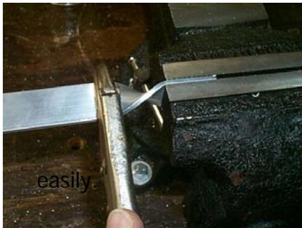
Take your 12" cut piece of flat aluminum and place about 1 1/4" of it in a vise. Using a pair of vise grip pliers, grip the aluminum about 1 1/2" away from the vise. Bend the Aluminum 90 degrees. I was shocked to learn how easy it was to bend using a vise and vise grips. Without these, I don't know how you'd bend it
