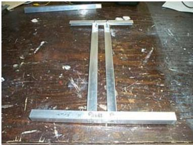
Now we're going to drill 2 holes in each section of angled Aluminum so they can be assembled as shown in the picture. This takes some calculation and some thought BEFORE DRILLING. Everything must be centered on itself. Let's go!
