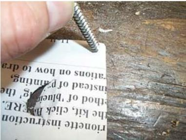
Cut out a square of the paper with the imprints the same size as the motor. Make holes in the center of the paper hole imprints using a knife or screw.
