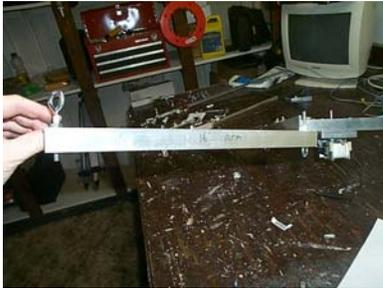
Put (2) eyebolts, (1) in each arm end using an eyebolt with nut screwed all the way on to act as a stopper and a nylon nut to secure it.
