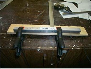
You can clamp the pieces together for drilling the first hole. A block of wood in between the 2 pieces of aluminum may help you to keep the Aluminum from shifting since they do not fit well together
