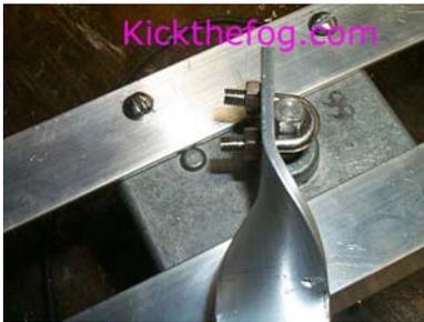
In the the picture, here, I have them tightened pretty good (Don't over tighten or you'll break the u-bolt!) and you can see the snug fit between shaft and u-bolt.
