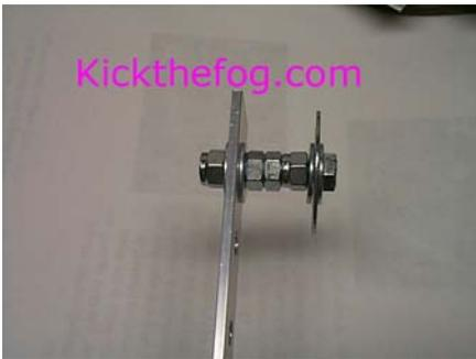
Assemble your crank end using the 1/4" X 1 1/2" Full thread bolt. I started in the outermost hole. This will give you the most movement. If later you decide your ghost is moving too much, you can move the full thread bolt in closer to the motor in one of the 2 other holes you drilled.
