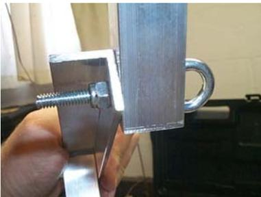
Then fasten them together using an Eye bolt with the eye pointed upward. *(the motor shaft points to the underside of the frame in case your having trouble knowing which side is up and which is down)* This eye bolt will be one of your mounting points from the ceiling. As you can see in the left picture, to assemble, you screw the regular nut that came with the eye bolt all the way on
