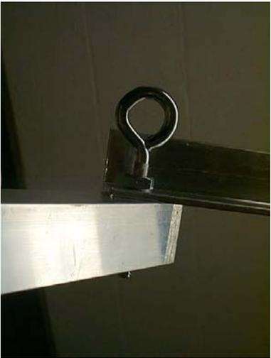
Let's mount the arms. Using your 1/4" drill bit, drill a hole at the edge of one of the arms. It doesn't really matter where. I measured a 1/2" in from the end and of course, 1/2" in from the side so the hole was in the center of the aluminum. Drill your hole there. Do the same thing for the ends of the 16" front piece.
