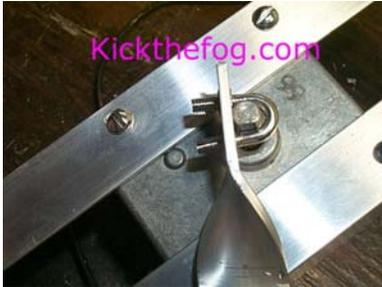
Place the crank we just built on the motor shaft so the Fender washer hangs down. Attach it to the motor drive shaft using the u-bolt and nuts. You'll notice that I placed the u-bolt so that it's inside edge rests firmly on the flat edge of the drive shaft. **THIS IS IMPORTANT** as to keep the crank from spinning around the shaft. We want the Motor shaft and Crank to become "one".
