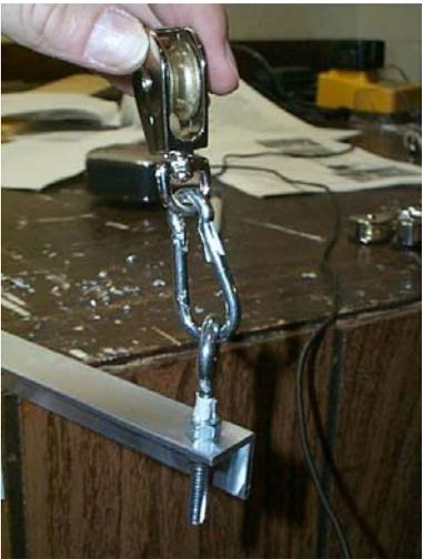
Note that the picture Here shows the installed pulley on the **BOTTOM** of the end of one arm (*frame is lying upside down*) (1) pulley on each arm end and (1) on the bottom center eyebolt of rear frame.
