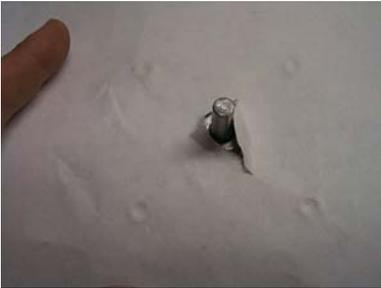
Time to mount the motor. I used a piece of paper and placed it over the motor shaft and pressed an imprint of the mounting holes into the paper. Look carefully and you can see the marks.
