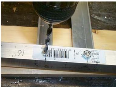
Now on the 16" front piece, from the outer edge you just marked, Measure inward 1/2" towards the center (half the width of the aluminum). This is dead center. Drill a hole with a 1/4" drill bit here. As you can see, I did the right side already and if you look closely you can see how I marked it and found my drilling locations on the front of my 16" piece.
