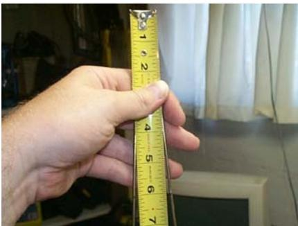
From the top of the hangar, measure down 6" and mark the hangar on each side.
