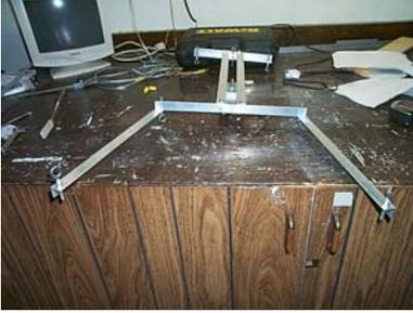
That's it...your frame it built! This gives you a pretty good look as to which eyebolts are pointing up and down. The 4 eyebolts on the frame face up. The 3 eye bolts, 1 on each arm end and the 1 in the center of the rear frame, face down.
