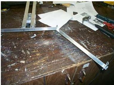
These eyebolts will be facing down (pointing same direction as the motor shaft) These will support your ghost's arms. Leave these nylon nuts just snug also so you can rotate it with some mild force also. Adjustment will be needed later.
