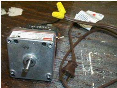
*(motor and extension cord already connected with wire nuts)*
