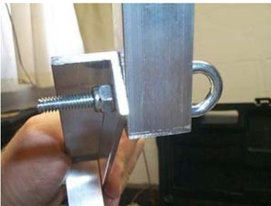
Then fasten them together using an Eye bolt with the eye pointed upward. *(the motor shaft points to the underside of the frame in case your having trouble knowing which side is up and which is down)* This eye bolt will be one of your mounting points from the ceiling. As you can see in the left picture, to assemble, you screw the regular nut that came with the eye bolt all the way on
