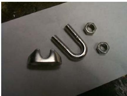
Disassemble your wire clamp. This is what we will use to mount the crank to the motor drive shaft. We are only interested in using the U-Bolt and the nuts. The other funny shaped part can be tossed.
