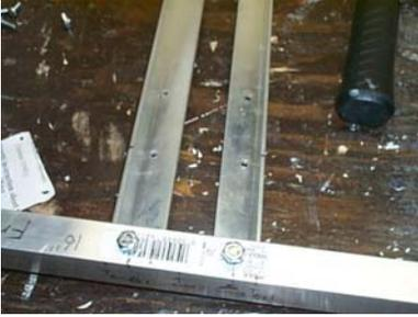
Drill the 4 holes you just marked with a 5/32 inch drill bit and enlarge if necessary. I had to enlarge mine with a 3/16 drill bit because I must have moved the paper a bit while marking (they didn't quite line up even with being able to move the aluminum)
