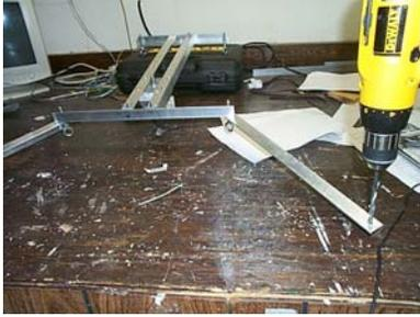
Here you can see in this bottom view of my frame that we have both arms secured to the frame using eyebolts. Now we must drill holes in the ends of the arms. Do this also with your 1/4" drill bit and center the hole on the end like you just did to mount the arms to the frame.
