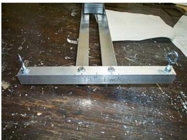
Turn your frame around. Drill and mount 2 more eyebolts the exact same way you did the others at the ends of the rear frame just like you did for the front. These will be pointing upward and will serve as the mount points to the ceiling.
