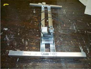
Use your (4) #10 X 1/2" bolts to secure the motor to the frame and tighten. Now you can go around and tighten all the other bolts/nuts and the frame will be nice and rigid. Do not over tighten or you will bend and flex the Aluminum and put extra stress on the little motor mount bolts.
