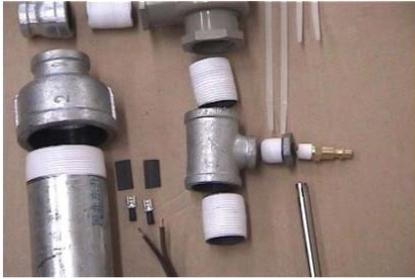
Next, let's get our air cylinder together. Be sure to use teflon plumber's tape on all the threads of the fittings and make sure all of your connections are very
