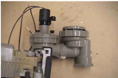
The shape of an anti siphon valve will give us a right angle exhaust to the inlet which makes our cannon very easy to use and to mount on the back side of walls with just the exhaust tip sticking out the other side. But first we will need to remove the unnecessary backflow device which can be done with a chop saw or jig saw as shown. Just cut between the two sides, just forward of the octagonal wrench fitting.
