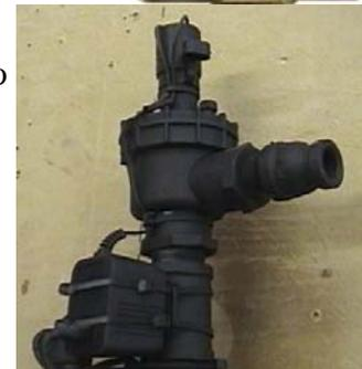
I simply used heat shrink tube to cover both of the legs and zip-tied the cords to the throat of the cannon. Then I used two heavy zip ties to attach the transformer to the side of the T fitting as shown here. If you look close you can see I used two more smaller ties, one on each side to keep the first ones from sliding off. This makes my cannon fully contained, and easy to transport.
