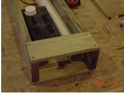
Next we started assembling the undercarriage. This had to be wide and deep enough to hide the fog machine and a pair of 2" wide steel pipe inside it, yet still look as realistic as possible.
