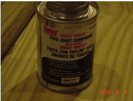
All pipes were sealed with the pipe joint compound pictured below - which we later discovered did a LOUSY job and leaked like crazy! We ended up pulling the whole thing apart and re-wrapping all the joints using a thick pink teflon tape. The thick tape worked great and everything was air tight and ready for battle!
