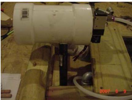
Below are some close-ups of the barrel assembly. The main area we're working with is the 4" PVC pipe with an angled 2" exit pipe.
