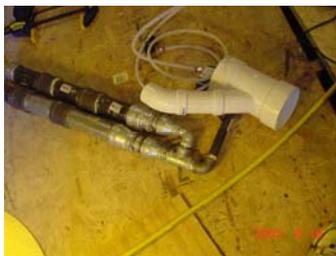
In the pictures above you can see a close-up of the whole pneumatic assembly (with shortened tanks for the time being). Air lines will feed into the nozzle bottom right to fill the tanks, and to another nozzle which will be attached to the valve (not pictured).
