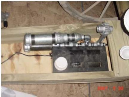
You can see above roughly how the pneumatics will sit in the cannon. I have 2 2" pipe (tanks) joined together at a 3/4" "T" fitting (the two pipes were used to maximize the amount of air we could "store" in the pipes to be released then the cannon "fires").
