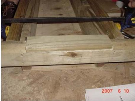
We also had to flatten the front lip of the axle so the side mounts that hold the barrel would sit evenly. These are pics of the notched front end.
