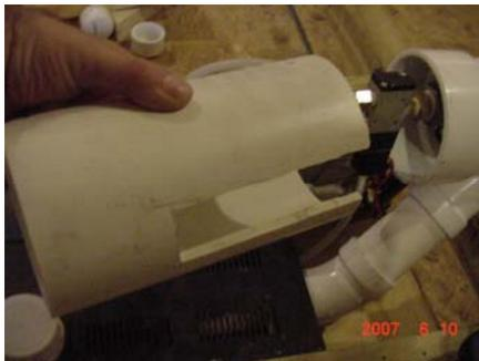
The valve assembly mounted on the back side of the QEV, and again because of the size of the valve, some creative carving/notching will have to be done to get the back end of the cannon barrel mounted.
