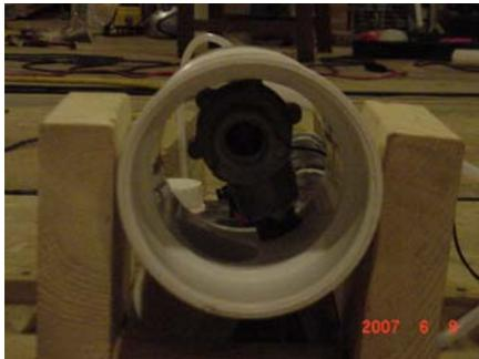
Because of the size of the QEV (it was too large to turn inside the PVC) I had to hold the QEV inside the PVC barrel and insert the black pipe up through the hole and twist to tighten it.
