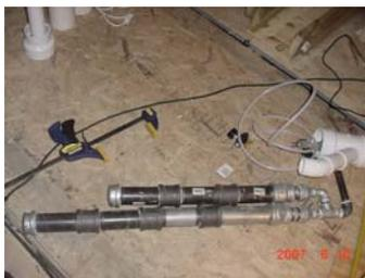
Here's a couple pictures of the assembled pneumatic assembly - tanks and valve (which had to be assembled inside the PVC barrel section).
