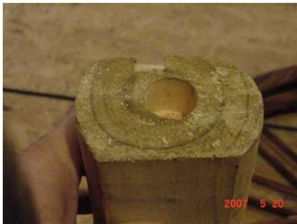
First we mounted the two wheels on a 4x4 axle. The wheels came with wood dowel inserts which we inserted into drilled out holes in the ends of the 4x4. After testing this we decided a sturdier axle was needed.
